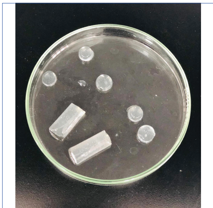
[Table/Fig-1]: Samples of tissue adhesive cut using a razor blade.
